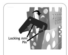
Pull the unit up until the locking arm fits over the pin on the side of the unit. 6
