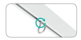
**b.** Slide the light hooks into the groove and place them in the center. Tighten Hook.
